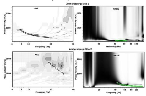
Figure 5. MSPAC-processed dispersion histograms from AVA recordings (left panels) and f-k-processed dispersion histograms from MASW recordings (right panels) generated for the two sites in Amherstburg. Open circles show manually picked dispersion estimates.
