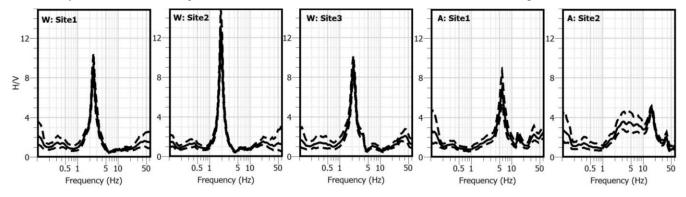
Figure 6. MHVSR curves from the ambient vibration array recordings for each of the five sites.
