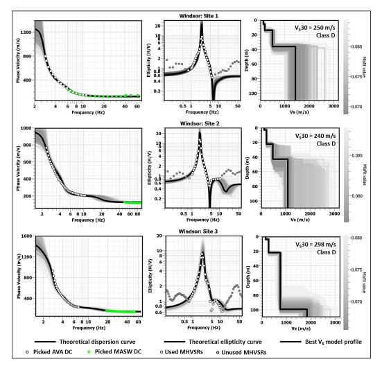
Figure 7. Joint inversion results for the three sites in Windsor. Input dispersion and MHVSR data are plotted as circles compared to theoretical dispersion and MHVSR curves (shaded lines) calculated from low misfit V<sub>s</sub> profiles (grey lines) and the minimum misfit Vs profile (black line).
