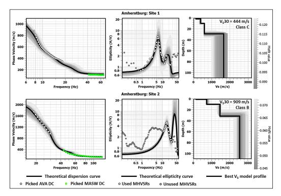
Figure 8. Joint inversion results for the two sites in Amherstburg. Input dispersion and MHVSR data are plotted as circles compared to theoretical dispersion and MHVSR curves (shaded lines) calculated from low misfit V<sub>s</sub> profiles (grey lines) and the minimum misfit Vs profile (black line).
